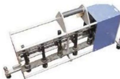
Figure 5 Typical tapping machines for impact sound insulation tests
