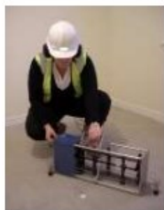
Figure 4 Impact sound test being carried out
